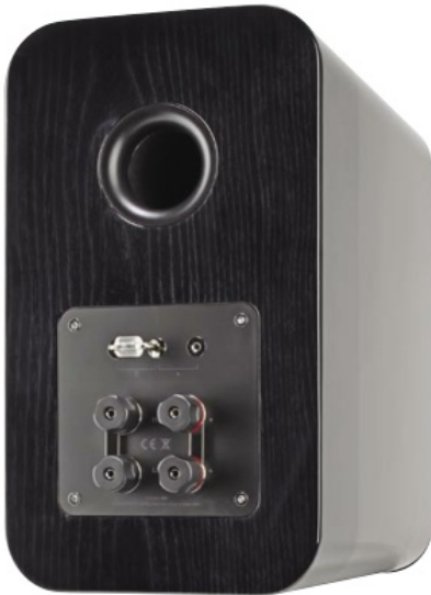
Two pairs of 'speaker binding posts allow for bi-wiring. A jumper connection alters frequency balance by +/- 0.5dB. Subtle but effective.
